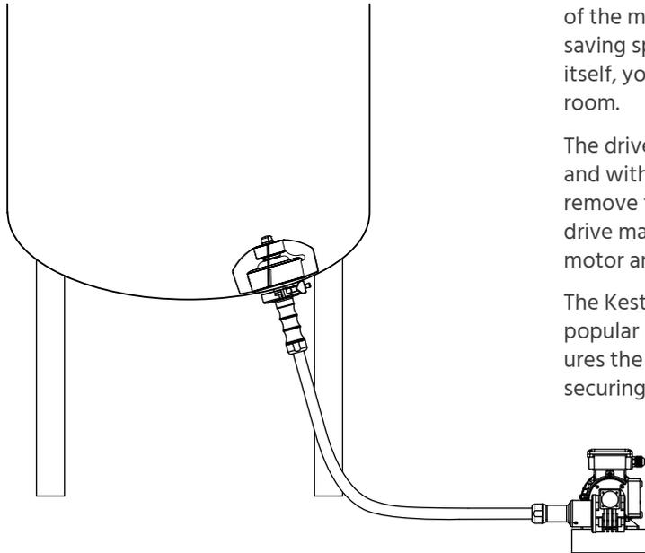
This new innovative drive unit allow you to get rid of the motor/gearbox from the tank. This is good for saving space and to remove the load upon the tank itself, you can even place the drive unit in a different room.
